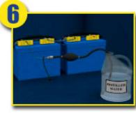
6. Begin pumping the squeeze bulb until it feels rigid. Your batteries are now filled to the proper level.
