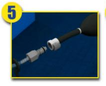
5. Connect the bulb pump to the fill line and Insert the other end into your container of distilled water.
