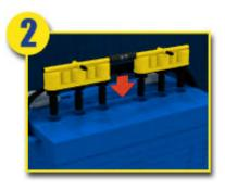
2. Remove vent covers and install manifolds assemblies into each battery.
