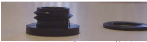
(Battery vent caps of Deka battery)
