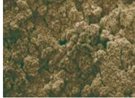
Lead Plate with No Sulfate Build Up
