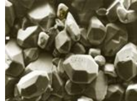
Lead Plate with Sulfate Build Up
